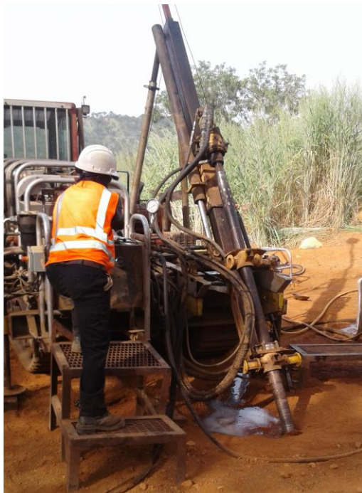
Diamond core drill in operation
